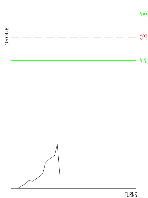
Figure 5: This graph indicates thread interference prior to seal engagement.
